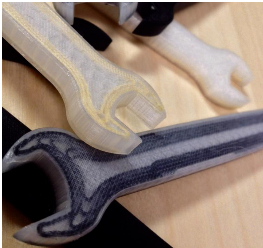
Nylon wrench reinforced with kevlar and carbon fiber
