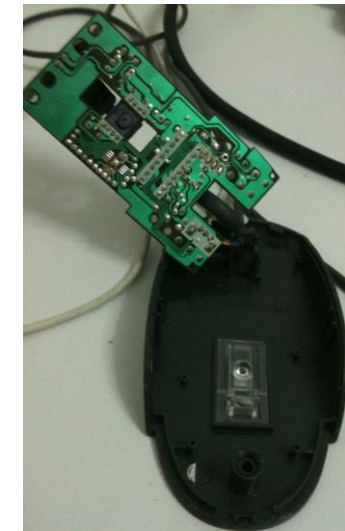
Fig. 2. A PCB in a computer mouse
