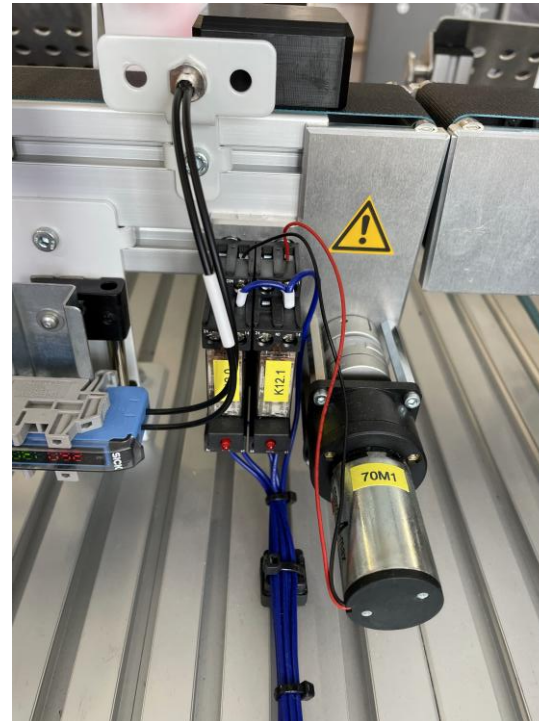
Conveyor belt with DC motor and light barrier
