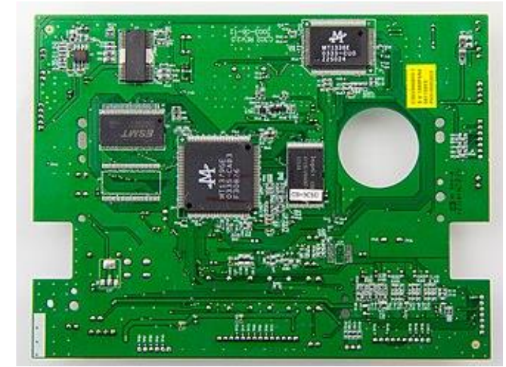
Fig. 1. Printed circuit board (PCB) of a DVD player
