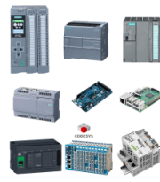
Supported devices: Siemens S7-300, S7-400, S7-1200, S7-1500, CODESYS V3 based PLCs, Raspberry Pi, Arduino-Due.
